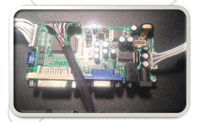
Notice the far left connector (gray ribbon cable) and the multi-way connector with the green wires.
